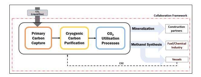
In the first stage of the CCUS system – Primary Carbon Capture. Membrane separation technology is currently limited by the selectivity of currently available membrane materials as well as the high cost of materials. One of the most promising gas separation method is using polymeric membrane that acts as the filter for the separation CO2/N2 mixtures and generates a specific gas rich permeate.
