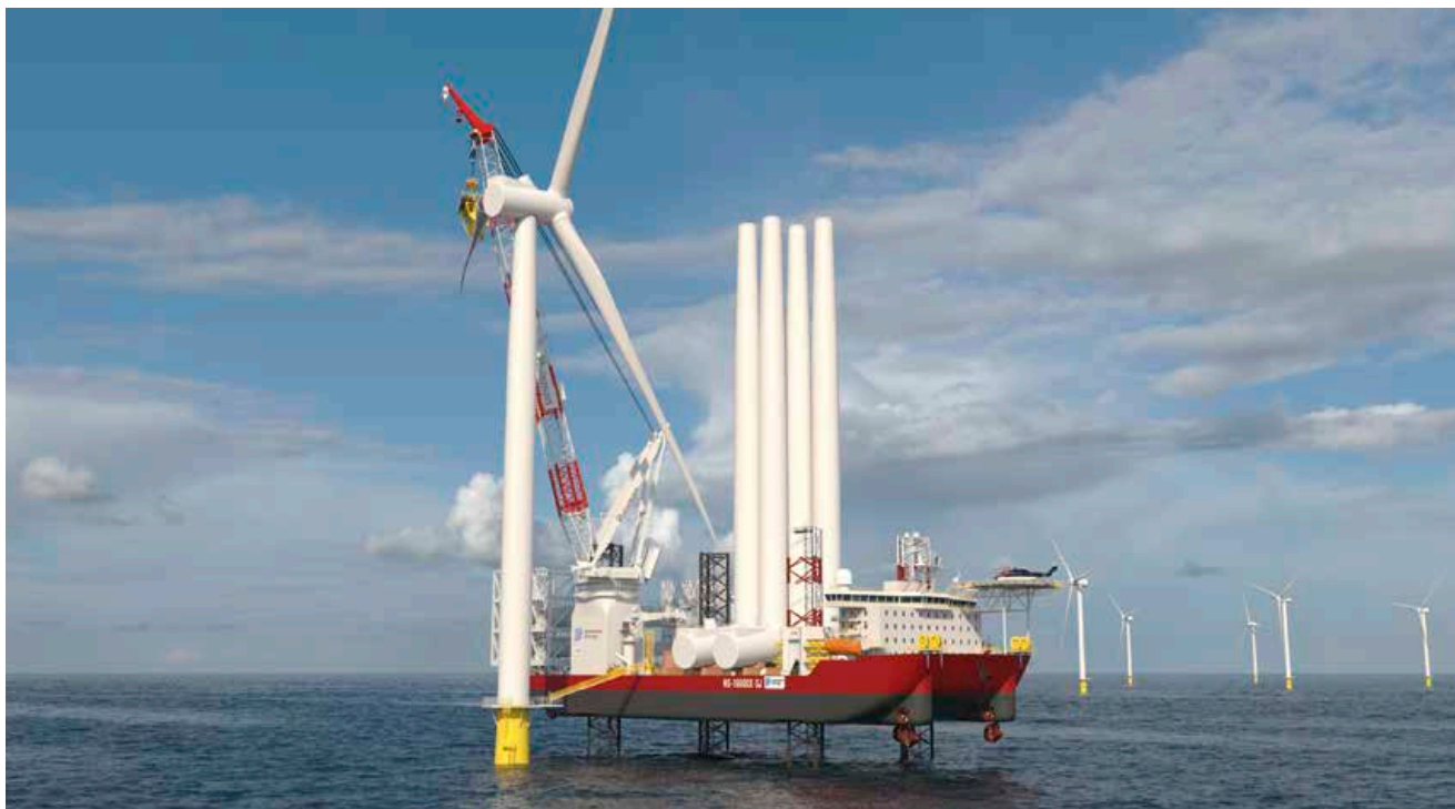
The vessel being developed for Dominion Energy Inc, named Charybdis, will be the first offshore wind turbine installation vessel in the United States and one of the largest vessels of its kind in the world.
