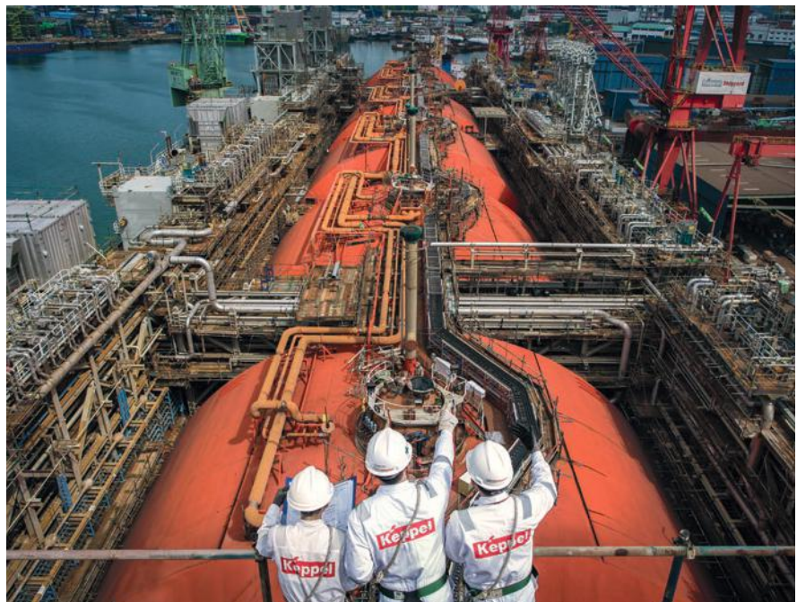
Golar Hilli, the world's first-of-its-type floating liquefaction vessel conversion, will be completed in 2017 for work in Cameroon.
