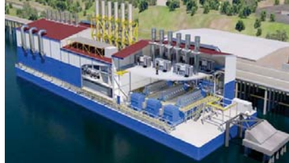
Single/Dual Fuel Floating Power Barge
