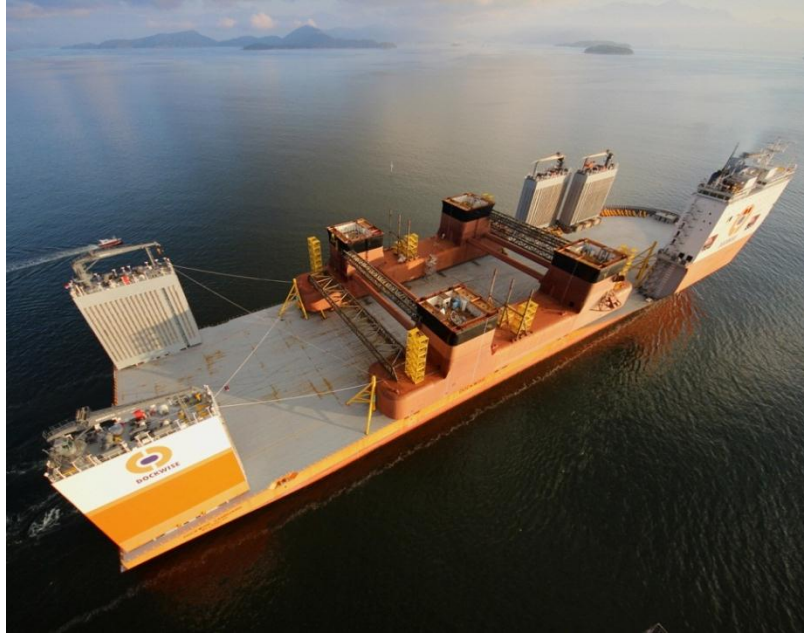
Lower hull of the first DSS™38E semi for Sete Brasil arrived safely at BrasFELS for integration with the remaining blocks
