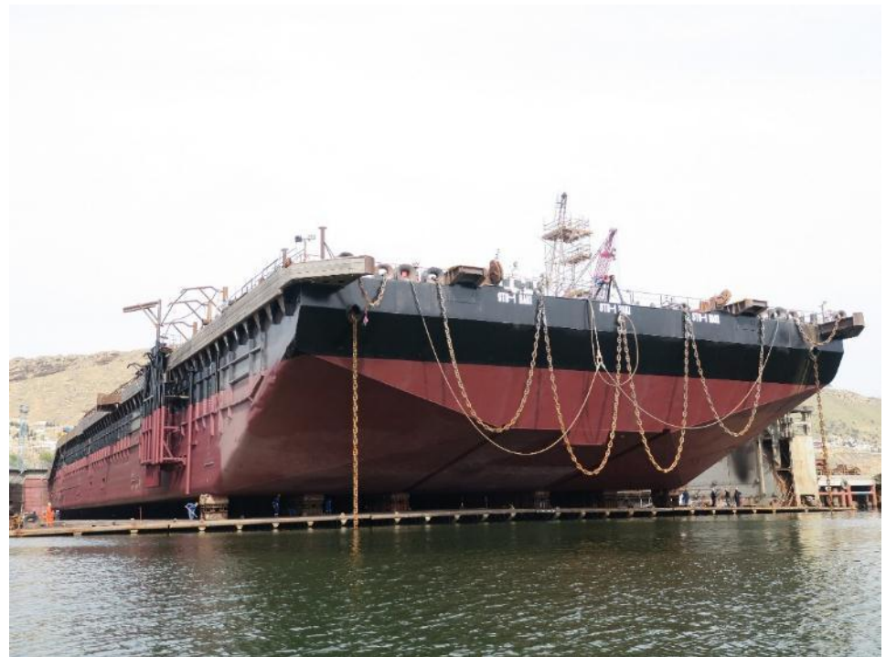
Purpose-built jacket transportation and launch barge, STB-1
