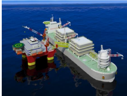
The first Floatel design with enhanced agility to follow a target such as a Turret Moored FPSO.
