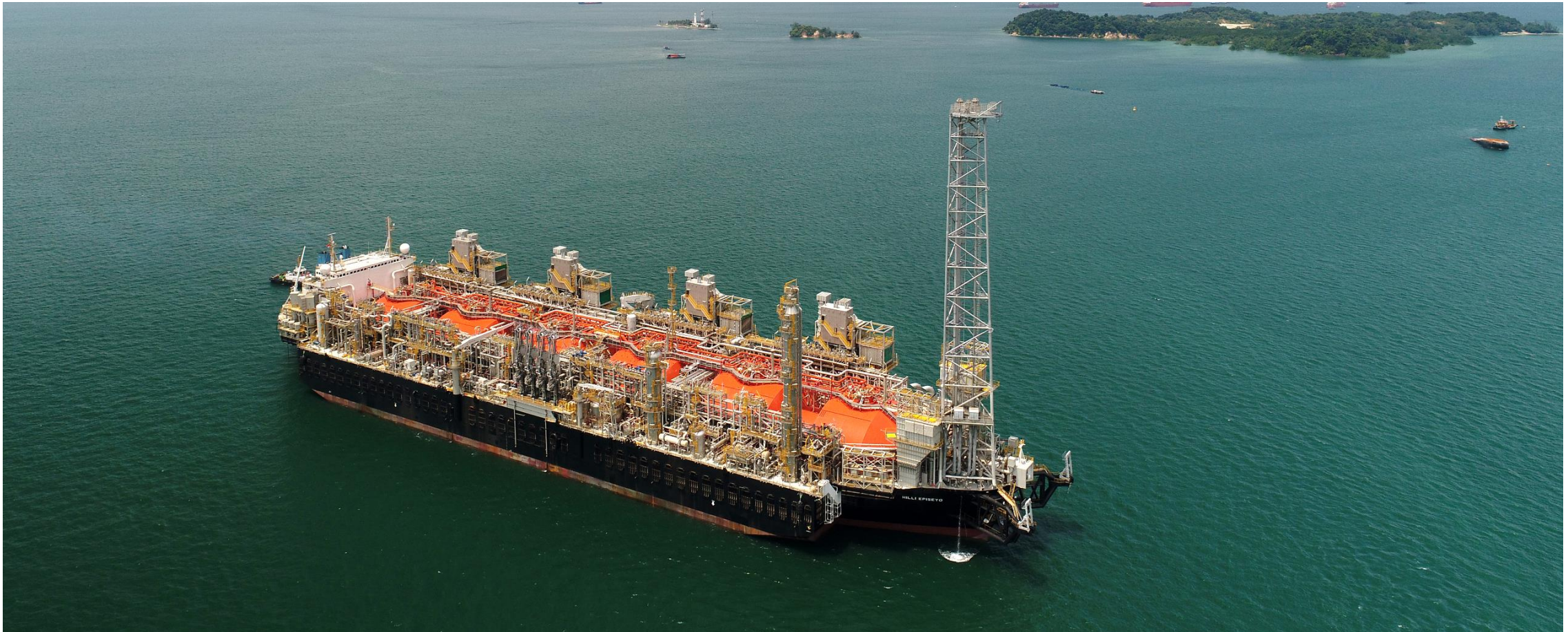
Golar Hilli Episeyo – the world's first converted FLNG vessel
